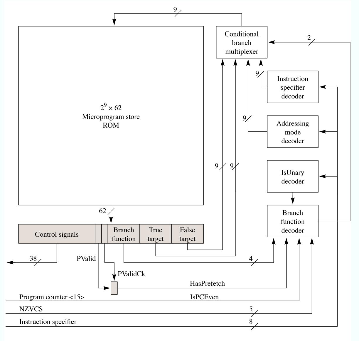
**Fig. 3** — The newly designed CPU control section.
