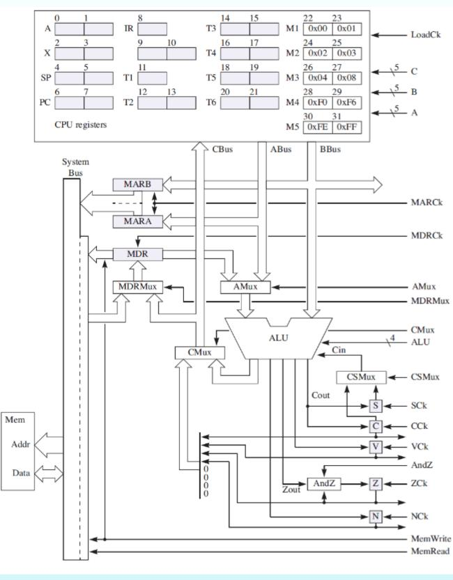
**Fig. 2** – Data section of Pep/9 CPU
